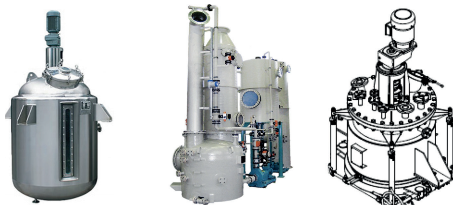
Fig. 22 – Reactor for dissolution in nitric acid (left), Scrubber for the utilization of nitrogen oxides (middle) and reactor for dissolution in sulphuric acid with oxygen (right).
