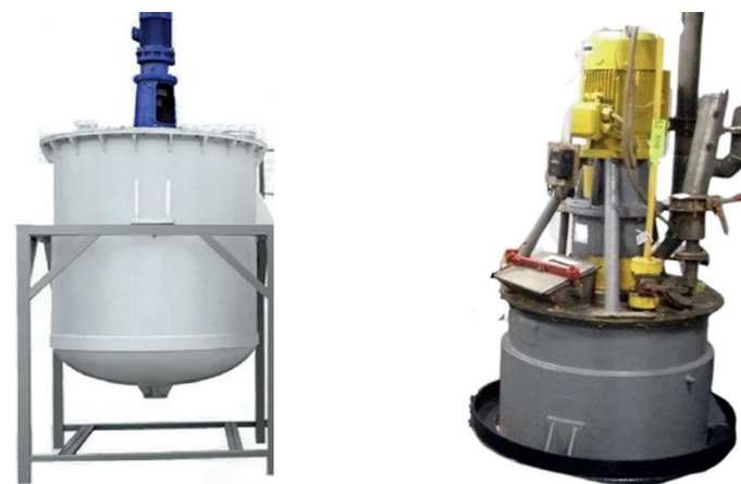
Fig. 12 – Polypropylene reactor (left) and titanium reactor (right).
